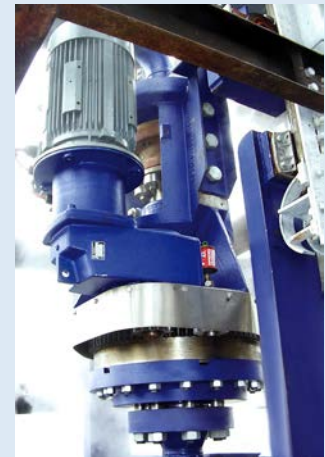
Drill Stem Drive, equipped with Electric Motor
