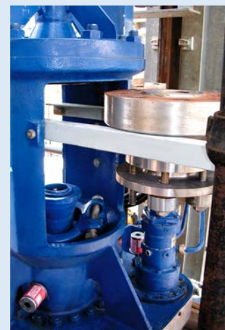
Cartridge design allows easily and Quick exchange Packing Cartridge
