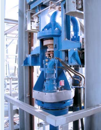
Drill Stem Drive, equipped with Hydraulic Motor
